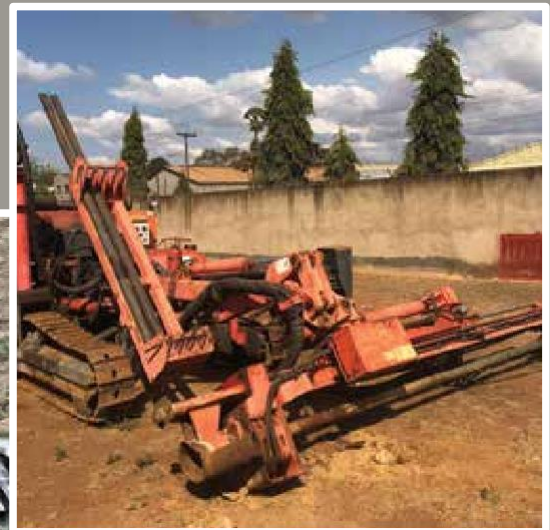
DRILLING RIG SANDVIK DI100 UP TO 120MM BIT
